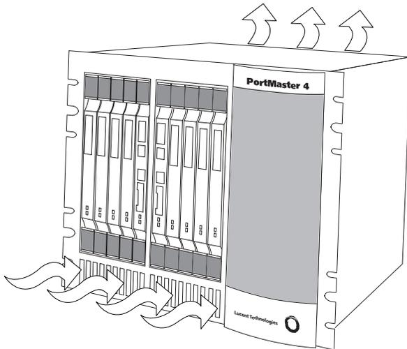
*The PostMaster 4 includes front-loading cards, field-replaceable cooling fans, advanced thermal design, and redundant hardware to maximize system uptime.*
