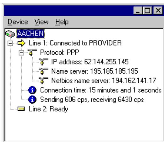
In this example, you can determine from the PPP protocol information the IP address assigned to your router by the provider for the duration of the connection and the addresses transmitted for the DNS and NBNS server.
