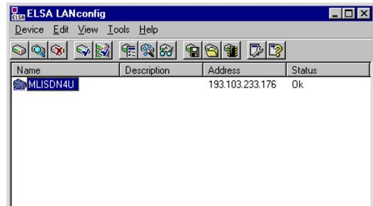
A number of queries will be made for the configuration of the *MicroLink ISDN 4U* for its first use. When you are asked for the IP address and network mask, enter the following values:
